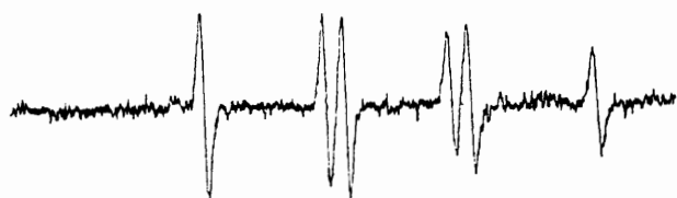
Fig. 3 EPR spectrum obtained on irradiation of SNAP in aqueous solution at pH 7 (1 G \equiv 2 mm)
